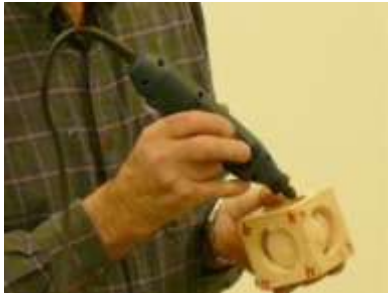
12. Tabs cut with carver or other cutting tool
