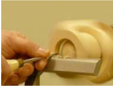
9. Continue to turn. Air gap beginning to show
