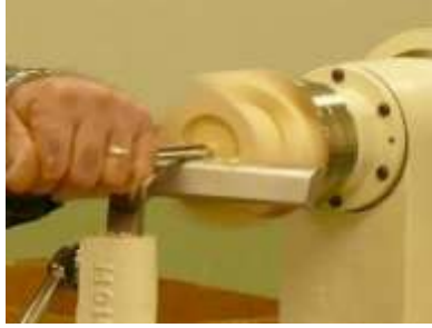
6. Topping off the sphere
